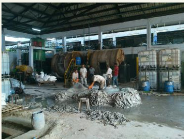
Hides being stacked following chrome tanning process ©WWF- UK/Conor Linstead
