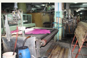
Leather coating and dyeing process ©WWF-Pakistan
