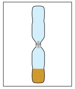
3. Attach the second bottle to the top of the first. Don't tape it all up yet, as you'll need to do some adjusting. Turn over the bottles and use your stopwatch to see how long the sand takes to flow. Put more or less sand in the first bottle until you reach as close to **four minutes** as you can. Then, seal up the join with the tape.
